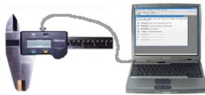
Figure 9: Example caliper connected to computer running JMP.
