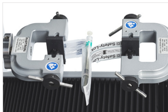
Figure 1. Image of Universal Testing Machine grips from Instron®. https://www.instron.com
