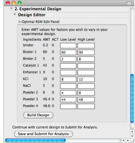
The virtual lab interface in JMP is a custom-made application built using JMP Scripting Language. The user identifies the factor levels so that the virtual lab can design an experiment, which SAS then runs.
