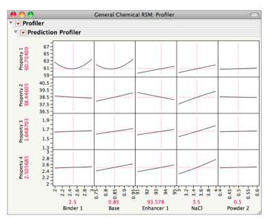
The Prediction Profiler in JMP enables virtual lab users to explore what-if scenarios quickly and easily. This example shows a predictive model. Users can change one factor (Binder 1, Base, Enhancer 1, NaCl, Powder 2) at a time and see the effect of that change on the predicted responses (Property 1, Property 2, Property 3, Property 4) and the interactions among the factors.
