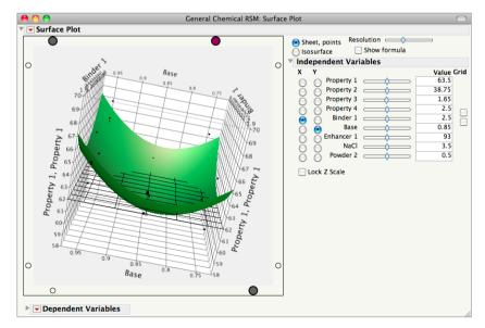
The JMP Surface Plot graphs points and surfaces in three dimensions. It enables users to examine the effect of two factors simultaneously. Users can rotate the plot and see relationships between the variables from all perspectives.
