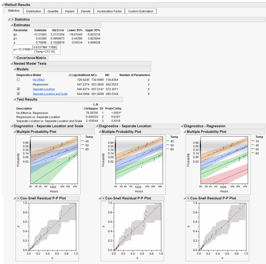
Figure 14.13 Weibull Distribution Nested Model Tests for Devalt.jmp Data
