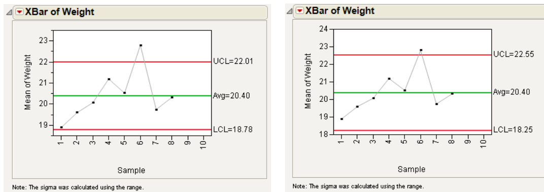
Figure 2.7 K Sigma =3 (left) and K Sigma=4 (right) Control Limits
