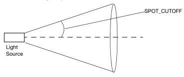
In addition to the cutoff angle, you can control the intensity and direction of the light distribution in the cone. SPOT\_DIRECTION specifies the direction for the spotlight to point; SPOT\_EXPONENT influences how concentrated the light is.
