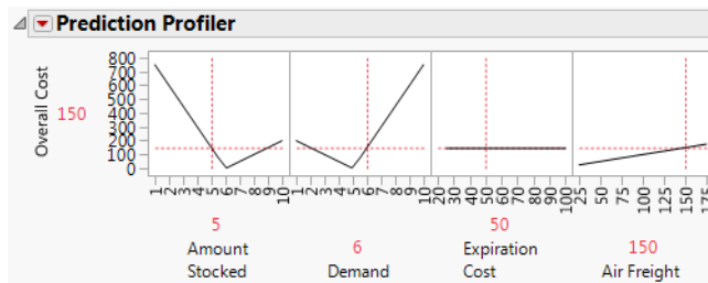
Figure 9.1 Example of a Prediction Profiler Using an Excel Model
